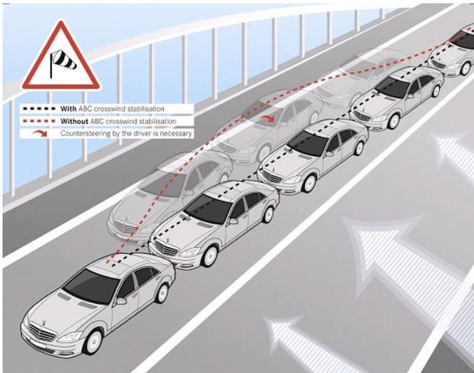
Fig. 3. Driving with and without stabilization function.
