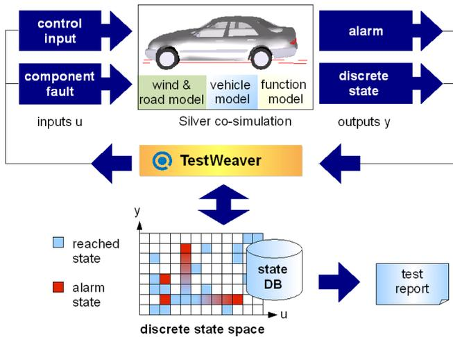
Fig. 1. Setup for simulation-based validation and test.
